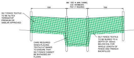
ELEVATION ON SILT FENCE AT DRAINAGE CHANNEL
